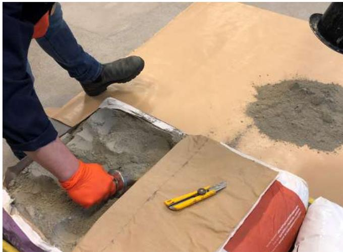
After 9, 12 and more than 18 months of storage, cement samples from two diagonally opposed quarters were taken and recombined. Copyright: EUROSAC/CEPI Eurokraft.
