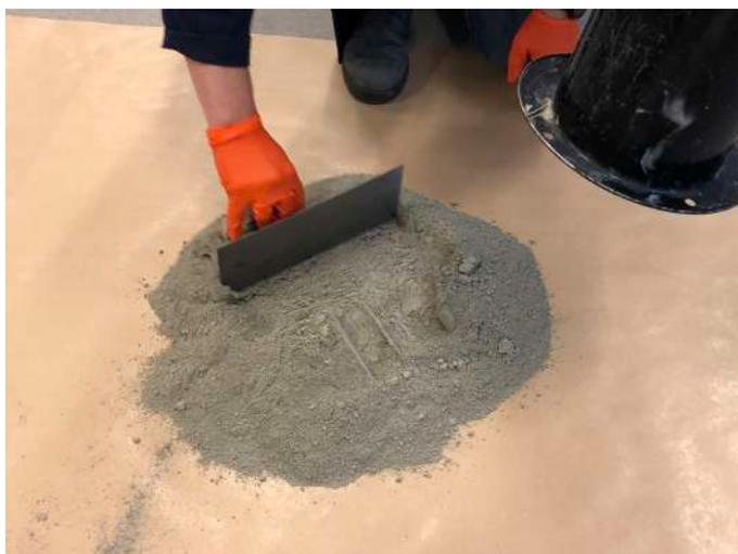
The cement samples were manually mixed before being sent to analysis. Copyright: EUROSAC/CEPI Eurokraft.
